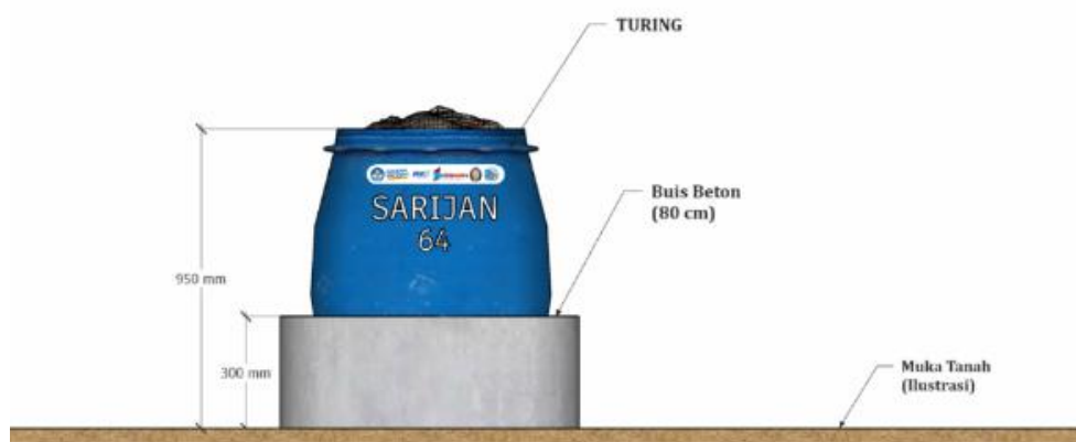
Figure 2. Illustration of the shape of TURING (net container barrel)
